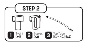
Insert four key no. 1 top tubes (3) into four T-joints, and two key no. 1 top tubes into two sockets. Make sure the holes in the tubes face the ground!
