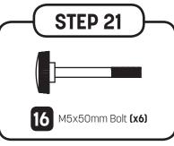
Next insert a curved tube (11) into the pole cap (14). Make sure the bent side of the enclosure poles are facing towards the center of the trampoline. Make sure the holes on the curved tube, pole cap, and strap ring are all aligned. Then insert a M5x50mm bolt (16) to secure in place. Important: Make sure the bolt goes into the round hole (not the hexagon hole) or you could break the pole cap! Repeat steps 20-21 to assemble the remaining pole caps.
