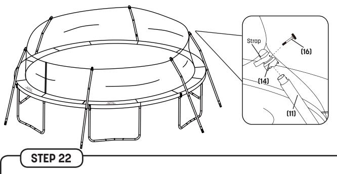
Starting from the enclosure door, lift one of the assembled poles and insert the straight tube (12) into the socket. Repeat this process to assemble the five remaining poles.
