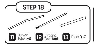
If you want, take a snack break because you're MORE THAN HALFWAY DONE, and you deserve it. This next step is easy. Just slide all the straight tubes (12) and curved tubes (11) into foam (13). If you're having trouble getting the foam over the tubes, try adding a small amount of water inside the foam!
