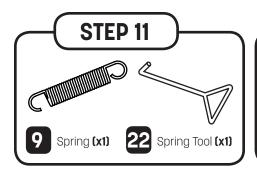
You may want to use gloves for this step! Before you begin, make sure the enclosure door is aligned with the T-joint just left of the warning label. Using the spring tool, hook the smaller end of a spring into the V-ring just left of the enclosure door. Stretch the free end of the spring until it reaches the frame hole on the corresponding T-joint.
