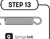
Next, place **four springs** on the **remaining four T-joints**. Make sure to **count the exact number of V-rings and frame holes** so each one corresponds!
