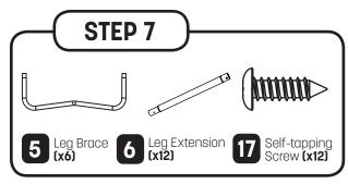
Insert two leg extensions (6) into one leg brace (5), and secure using two self-tapping screws (17). The peak of the leg brace should point upwards. Note: Make sure not to confuse the leg brace with the curved tube. Repeat this step to complete six leg sections.
