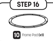
Place the frame pad **(10)** on **top of the springs**. Adjust the frame pad so that the **slits are** directly **above the T-sockets**, and the **two logos are on either side of the enclosure door**.
