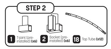
Insert the large side of a top tube (18) into a T-joint (1). Then insert another top tube (18) into a socket (2). Now slide the top tube (18) with T-joint (1) onto the small end of the top tube with socket (2) making one frame section.
