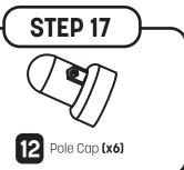
Important: The pole cap (12) has two sides; one with a hexagon hole, and one with a regular hole.
