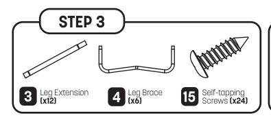
Insert a leg brace (4) into two leg extensions (3) and tighten with two self-tapping screws (15). Now insert both leg extensions (3) into a T-joint and socket of a frame section at the same time. Tighten with two self-tapping screws (15). Repeat this step until you have six frame pieces assembled.
