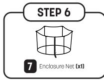
Now place the enclosure net (7) on the jump mat (5), and make sure the first hole (the hole directly to the left of the enclosure door zipper) and the first V-ring (the V-ring directly to the left of the warning label) line up. Now insert the first V-ring into the first hole. Then, insert the remaining V-rings into their corresponding holes. Once you've finished, the enclosure net should be fully attached to the jump mat.
