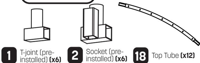
Insert the large side of a top tube **(18)** into a T-joint **(1)**. Then insert another top tube **(18)** into a socket **(2)**. Now slide the top tube **(18)** with T-joint **(1)** onto the small end of the top tube with socket **(2)** making one frame section.
