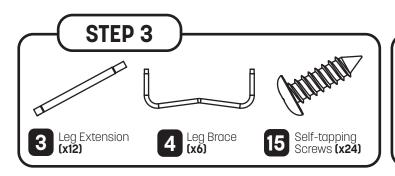
Insert a leg brace (4) into two leg extensions (3) and tighten with two self-tapping screws (15). Insert both leg extensions (3) into a T-joint and socket at the same time, and tighten with two self-tapping screws (15). Repeat this step until you have six frame pieces assembled.
