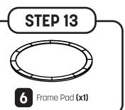
Place the frame pad **(6)** on **top of the springs**. Adjust the frame pad so that the **slits are** directly **above the T-sockets**.
