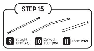
If you want, take a snack break because you're MORE THAN HALFWAY DONE, and you deserve it. This next step is easy. Just slide all the straight tubes (9) and curved tubes (10) into foam (11). If you're having trouble getting the foam over the tubes, try adding a small amount of water inside the foam!
