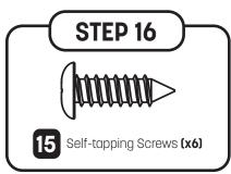
Insert one straight tube (9) into one curved tube (10), and secure with one self-tapping screw (15). Important: On the curved tube there is one end that has two holes. Make sure that end is on top!
