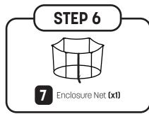
Now place the enclosure net **(7)** on the jump mat **(5)**, and make sure the first hole *(the hole directly to the left of the enclosure door zipper)* and the first V-ring *(the V-ring directly to the left of the warning label)* line up. Now insert the first V-ring into the first hole. Then, insert the remaining V-rings into their corresponding holes. Once you've finished, the enclosure net should be fully attached to the jump mat.
