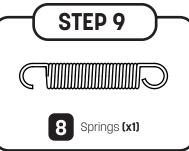
Now, **repeat step 8** on the **other side** of the trampoline. Attach the small end of the spring just **left of the warning label and** stretch the free end of the spring until it reaches the **frame hole** just **left of the T-joint**.
