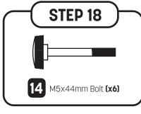
Next insert a curved tube **(10)** into the pole cap **(12)**. Make sure **the bend** of the enclosure poles are **facing out away from the center** of the trampoline. Make sure the holes on the curved tube, pole cap, and strap ring are all aligned. Then insert a M5x44mm bolt **(14)** to secure in place. **Important: Make sure the bolt goes into the round hole (not the hexagon hole) or you could break the pole cap!** Repeat steps 17-18 to assemble the remaining pole caps.
