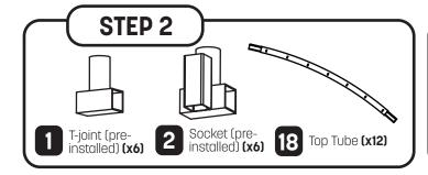
Insert the large side of top tube (18) into a T-joint (1) and insert another top tube (18) into a socket (2). Then insert one top tube (18) with T-joint (1) into one top tube with socket (2). Make sure the holes in the tubes face the ground! Now repeat this step for the remaining top tubes with T-joints and top tubes with sockets. Make sure the T-joints and sockets are alternating!
