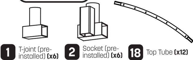
Insert the large side of top tube **(18)** into a T-joint **(1)** and insert another top tube **(18)** into a socket **(2)**. Then insert one top tube **(18)** with T-joint **(1)** into one top tube with socket **(2)**. **Make sure the holes in the tubes face the ground!** Now repeat this step for the remaining top tubes with T-joints and top tubes with sockets. **Make sure the T-joints and sockets are alternating!**
